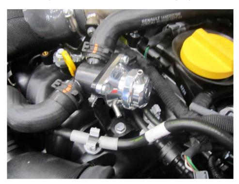
10. The boost pipe on top of the engine needs to be moved over to allow you to run the new silicone vacuum hose for the Forge valve. Undo the 10mm fastener that holds the boost pipe to the engine, then unclip the hose clamp with the use of a flat blade screw driver. You will then be able to pull the boost pipe off the turbo and move it over to the left side of the engine bay.
