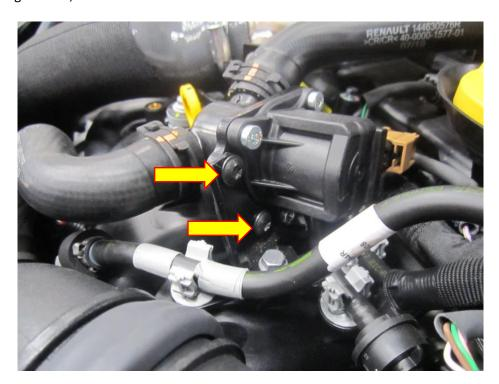
2. With the OE valve freed from its bracket you will now be able to access all three 4mm Allen fasteners which need to be removed with a 4mm Allen key/socket attachment. Unclip the brown plug on the valve by pushing down on the tab at the back, with that removed the OE valve will come away from the vehicle.
