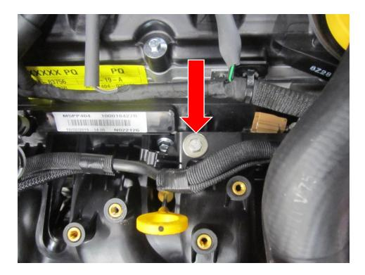
7. Mount the solenoid from the kit as shown in the picture, replace the 10mm fastener you have removed with the M6x20 fastener and M6 washer provided with the kit.
