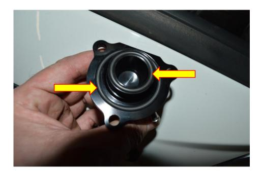
9. Fit the new Forge Motorsport valve in place where the OE valve was fitted. Use the original fasteners to hold it in place. Do not fit the two T30 Torx fasteners just yet.
