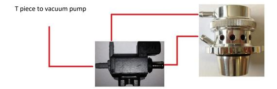
12. Run the new vacuum lines as per the previous step and cut to length with some side cutters or a sharp blade. The hose which runs to the T piece runs under where the boost pipe is located. Use the supplied cable ties to secure the ends of the vacuum lines to the solenoid, valve and vacuum T piece, then snip off the excess with side cutters.
