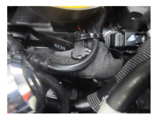
16. Refit the boost pipe, push the end of the hose back into the turbo, make sure you hear a positive click when pushing it in, then replace and tighten the 10mm fastener that holds the boost pipe to the engine.
