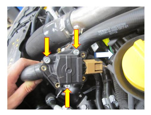
3. Locate the vacuum hose for the brake servo, this is just in front of the OE valve near the front of the engine bay. There is a metal hose clamp that needs to be removed, use a flat blade screw driver to open the clamp. With the clamp opened, separate the rubber hose from the plastic joiner.
